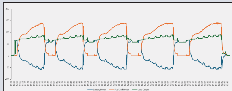
VARIABLE POWER 50 kW Charger Running for 3 Hours. Switching Between Fuel Cell and Battery System.
